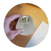
Screw bolts into base of detacher. Thread nuts onto bolts and screw up from underneath the POS until tight.
